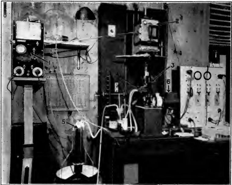
FIG. 3. Apparatus set-up for taking motion pictures of microscopic phenomena at very low temperatures. (1) Camera timer with motor, (2) camera, (3) microscope, (4) freezing chamber on microscope, (5) freezing apparatus, (6) light-source
